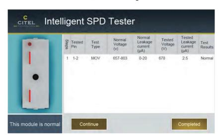
Figure 5-9 Screen displayed after the test is completed
