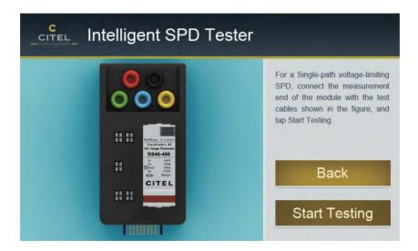
Figure 5-6 Testing a plug-in module
