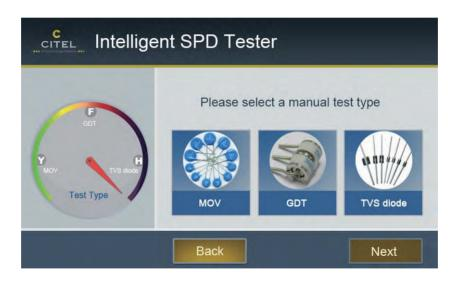
Figure 5-10 Manual test type selection screen
