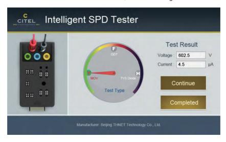
Figure 5-14 Display of the test result for a manual test type
